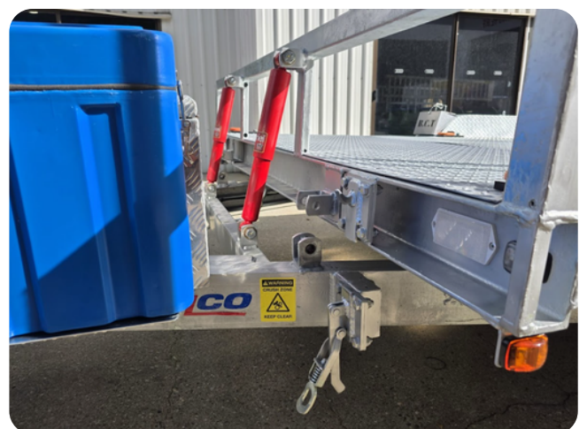
Manual tilt drawbar with cam locks
